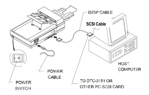
Figure 2-8 Scanpartner 15C Scanner Cable Connection
